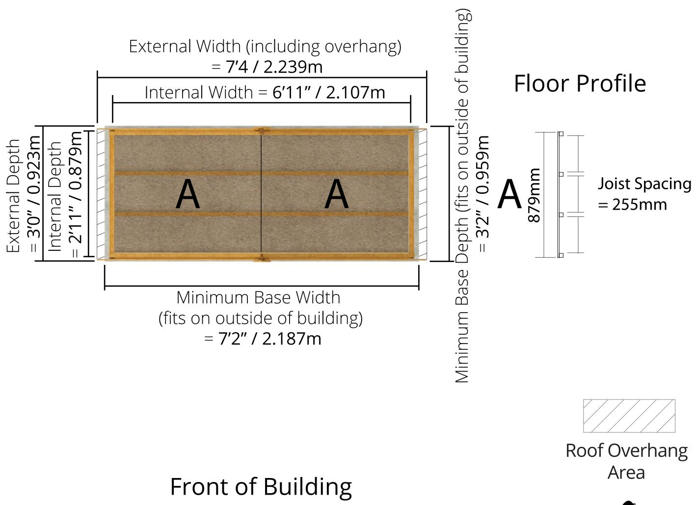
Please note: your base must be solid and perfectly level with drainage to allow water to run off the surface. There must also be a suitable clearance on each side to allow annual treatment to be applied.
