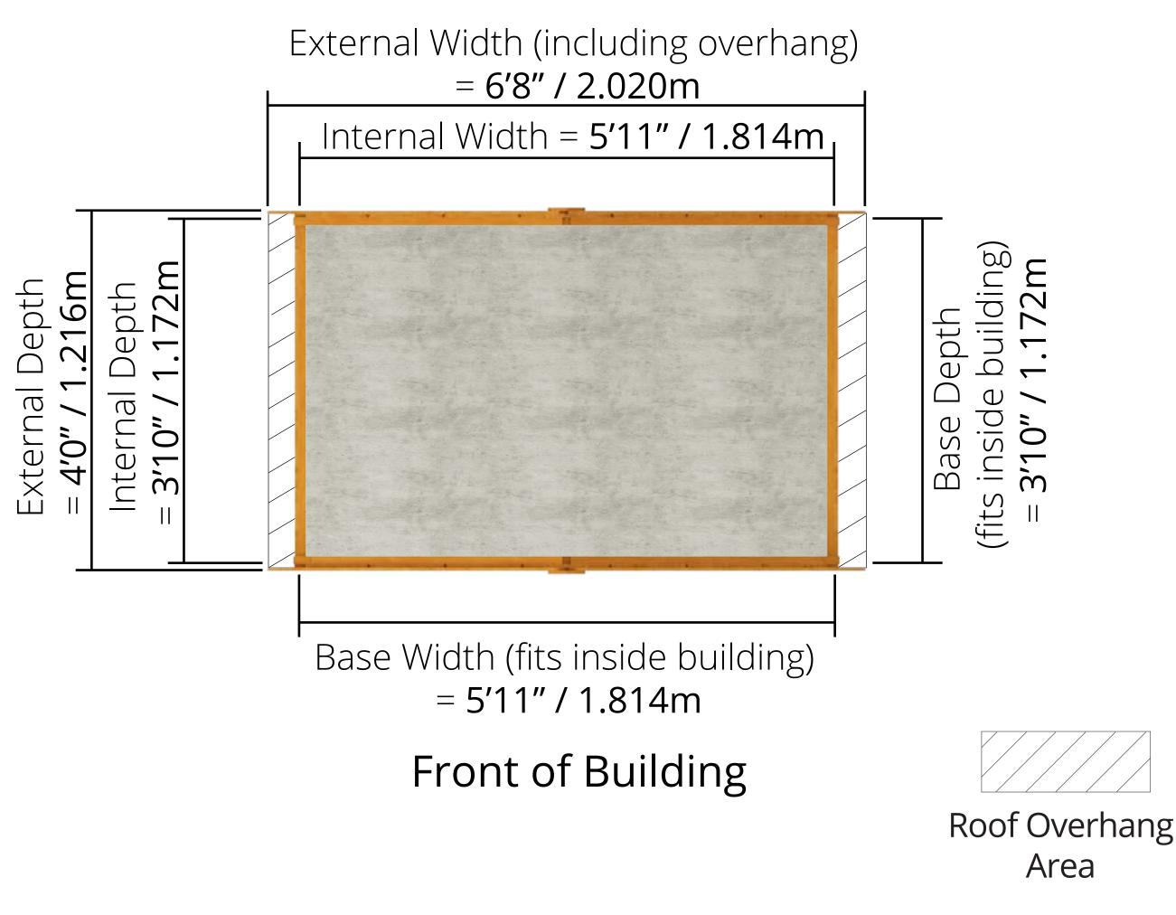
Please note: your base must be solid and perfectly level with drainage to allow water to run off the surface. There must also be a suitable clearance on each side to allow annual treatment to be applied.
