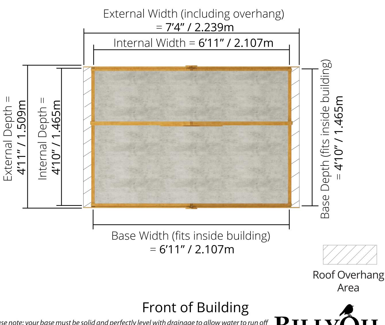
Please note: your base must be solid and perfectly level with drainage to allow water to run off the surface. There must also be a suitable clearance on each side to allow annual treatment to be applied.
