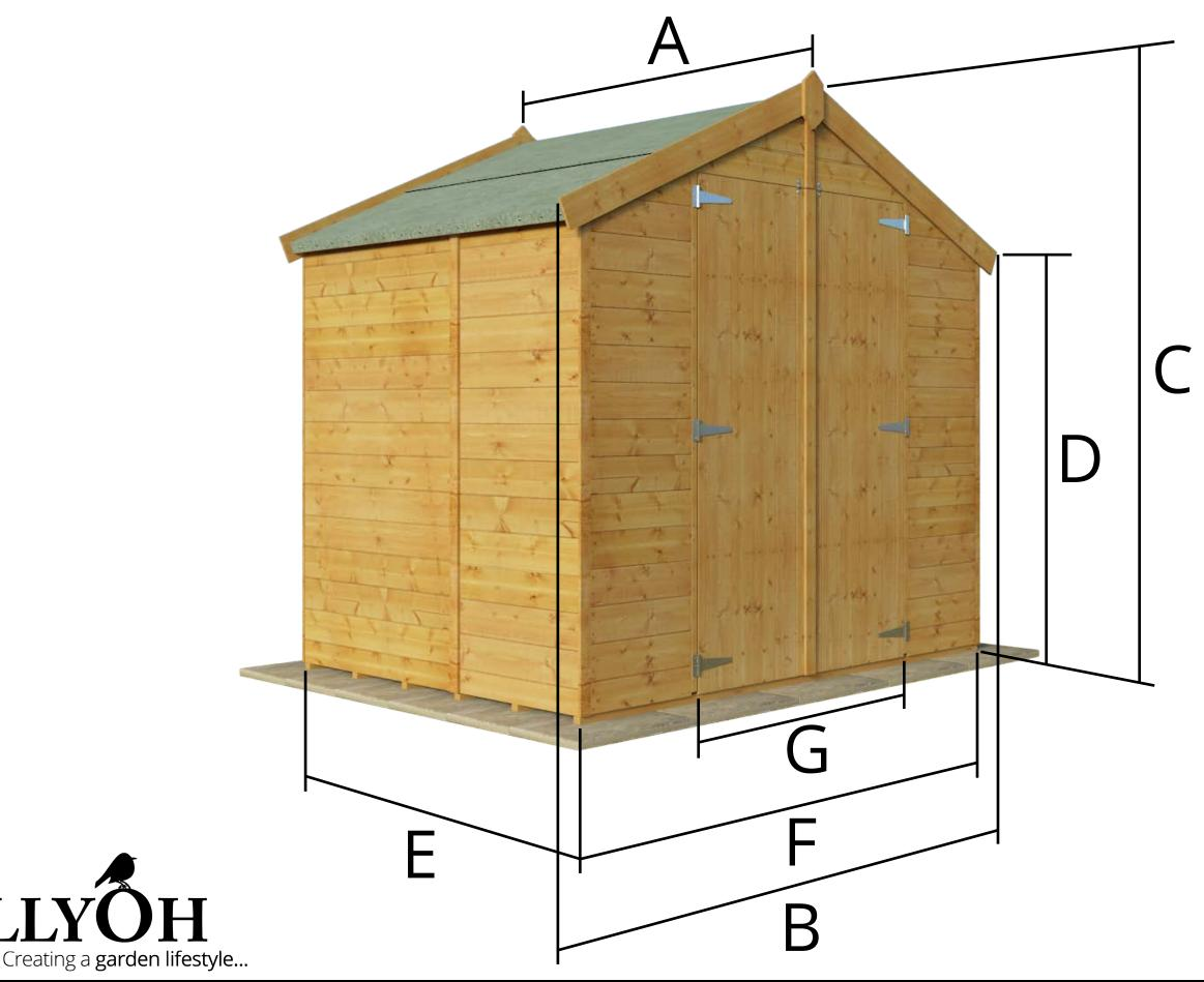
A: Overall Building Depth (including overhang) = 4'11" / 1.509m B: Overall Building Width (including overhang) = 7'4" / 2.239m C: External Ridge Height (including floor) = 6'8" / 2.035m D: External Eaves Height (including floor) = 5'1" / 1.549m E: Total Floor Depth = 4'9" / 1.465m F: Total Floor Width = 6'11" / 2.105m G: Door Opening Width = 3'8" / 1.118m
